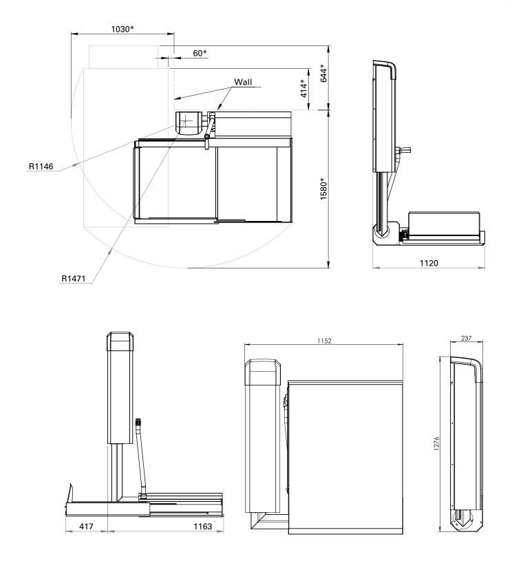
$<sup>\</sup>mbox{^*}\mbox{Dimensions}$  depend on wall bracket and façade. May differ from installation to installation.
